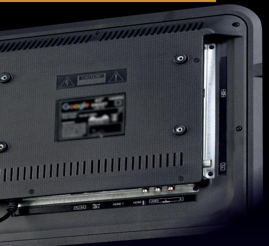
Port HDMI 2.0x2 USB 2.0X2 Ethernet AV Input Optical COAX Headphone Jack
